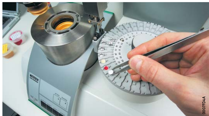
Figure 1 Analysis of the thermal behaviour of greases
